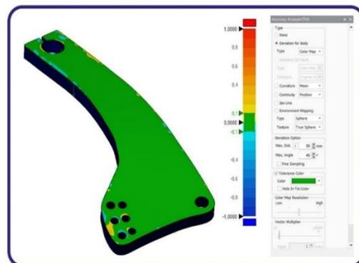
Figure 7. Deviation analysis results between mesh and solid model
