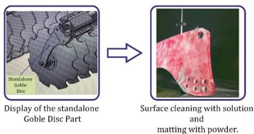
**Figure 2.** Preparing the agricultural machine part for 3D scanning
