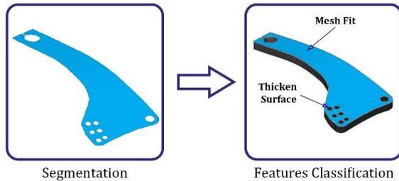
Figure 4. Applying segmentation and feature classification processes to the agricultural part
