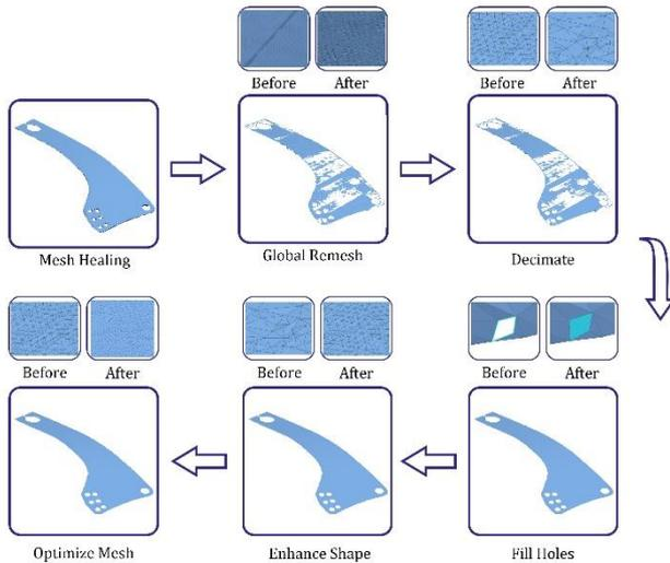
Figure 3. Data processing flowchart in reverse engineering
