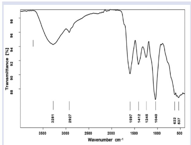
Figure 6. FT-IR spectrum of carbon quantum dots synthesized from *M. sylvestris*.
