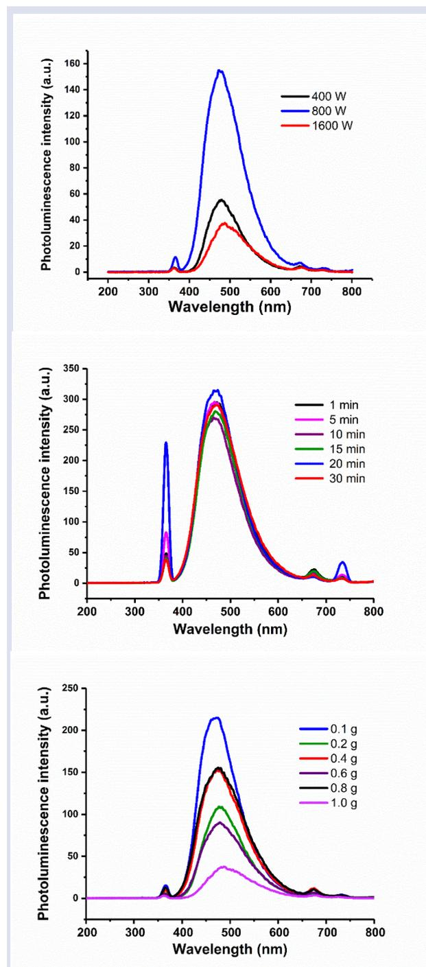
Figure 1. Optimization of operational parameters for synthesizing CQDs from *M. sylvestris* through microwave irradiation (Microwave power level: 800 W, exposure time: 20 min, the mass of *M. sylvestris* plant powder: 0.1 g and the volume of distilled water: 10 mL).
